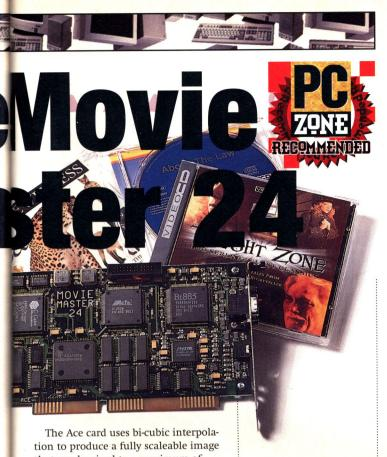
The Ace card uses bi-cubic interpolation to produce a fully scaleable image that can be sized to a maximum of 1280x1024. This produced some of the highest quality MPEG playback we've seen so far, with very little colour banding or picture degradation. Interpolation works by grading between different colours, so instead of getting a line where two colours meet you get a smooth merging.
