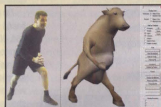
Paul's attempts to walk like an angry giant cow (left) have been captured on video. The 3D cow (right) is modelled to mimic his movements, frame by frame.
