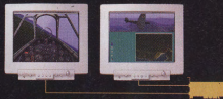
One AGP card supports two displays
